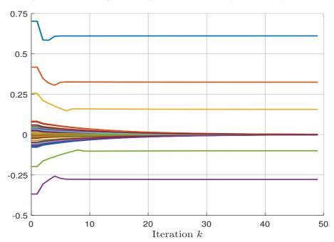
Figure 3: ADMM algorithm applied to the lasso optimization problem
